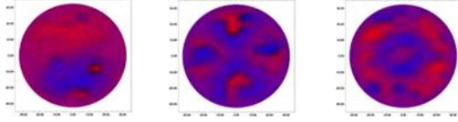
Mode (1,1), 140 Hz    Mode (2,1), 210 Hz    Mode (0,2), 226 Hz
