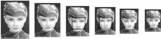
Fig. 2- Scanning window is applied to the entire image in different scales
