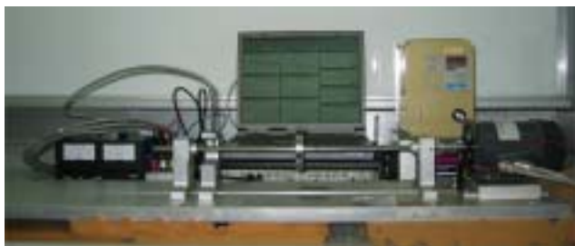
Fig.1 Unbalanced rotor and loose base system of the experiment rotor kit.
