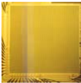
Fig.6 The photo of 128x128 test socket chip
