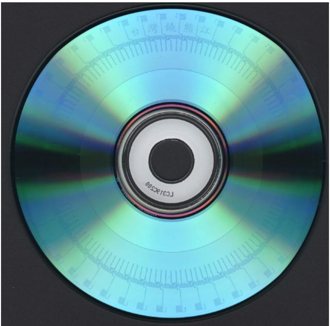
Fig. 3. The scanner image of centrifugal microfluidic lab-on-a-CD system for multiple enzymatic assays and digital information imprinted on CD-R using CD-Recorder. For demonstrating the potentials to integrate microfluidic structures and digital information on the same CD-R platform using CD-Recorder, patterned on outer layer, the microfluidic structure was chosen with the centrifugal microfluidic system design for multiple enzymatic assays [10]; encoded on inner layer, the digital information was demonstrated with a piece of music “Air” from the “Water Music Suite”. Also, for decreasing the effects of light reflecting and improving the quality of image capturing, image was taken by using PC scanner but not digital camera.
