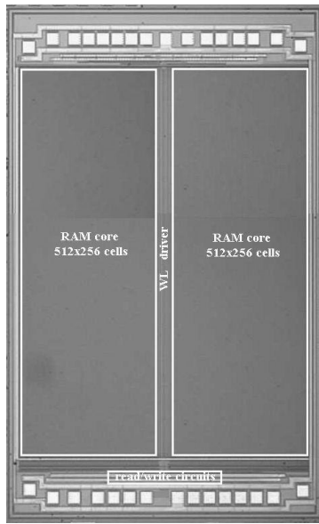
Fig. 11 A photomicrograph of 32Kx8 SRAM
