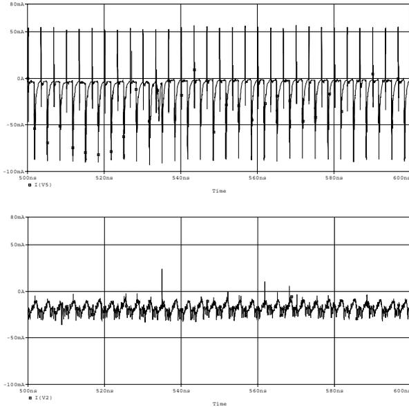
Fig. 7. Current from power supply line for a single clock (above) and the proposed alternative (below).
