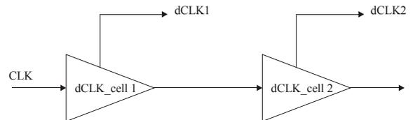
Fig. 3. dCLK\_cell chain for clock generation
