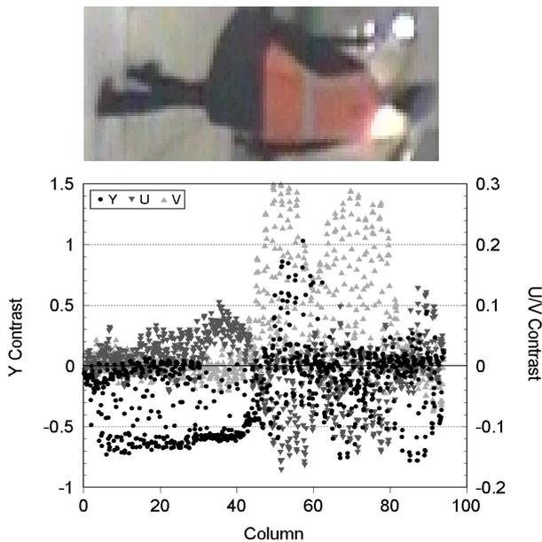
Fig.4 Contrast plot of pixel within a blob comprising a person wearing a bright orange waistcoat –negative U contrast for yellow and positive V contrast for red- with a grey band in the middle.
