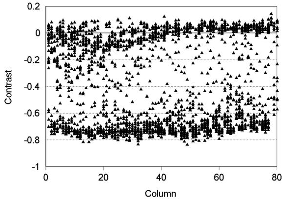
Fig.2. Effect of changes in illumination conditions: luminance contrast of background pixels shifts to positive values. The cloud of pixels with low negative contrast (columns 0 to 40) is associated with the shadow of the person.
