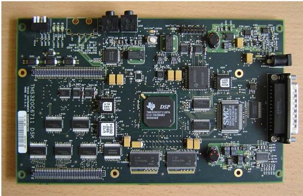
Figure 1: TMS320C6711 DSK board for OFDM modulator and demodulator implementation.
