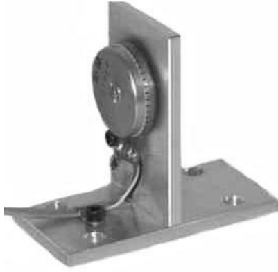
Figure 5: View of the piezoelectric motors used [6]
