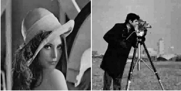
Fig. 2. Lena (PSNR = 27.6 dB, 0.21 bpp) and Cameraman (PSNR = 24.37 dB, 0.21 bpp) using proposed method.
