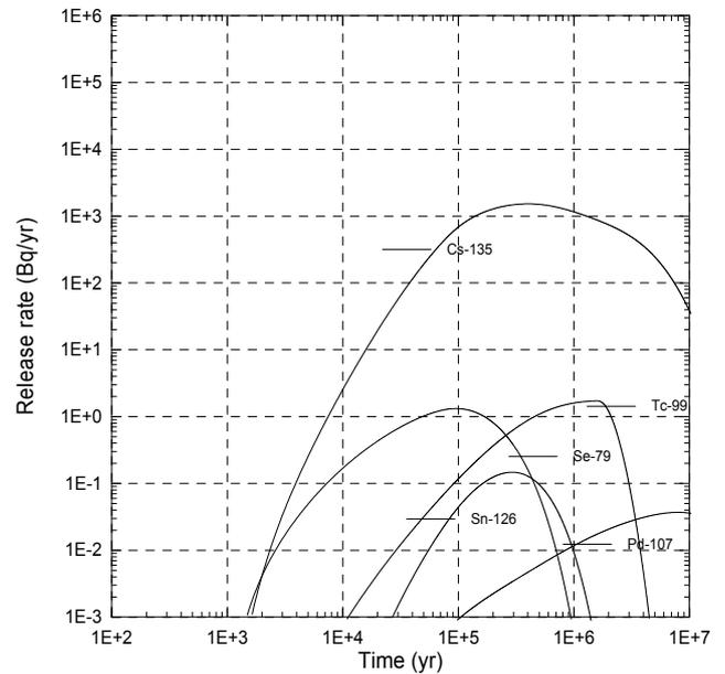
Fig. 2. Release rate of fission products from the host rock to the MWCF per waste package
