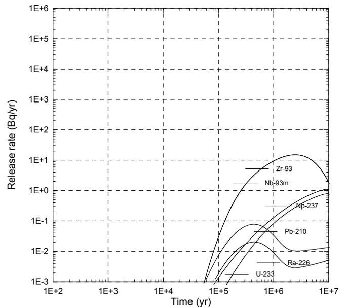
Fig. 3. Release rate of decay chains from the host rock to the MWCF per waste package
