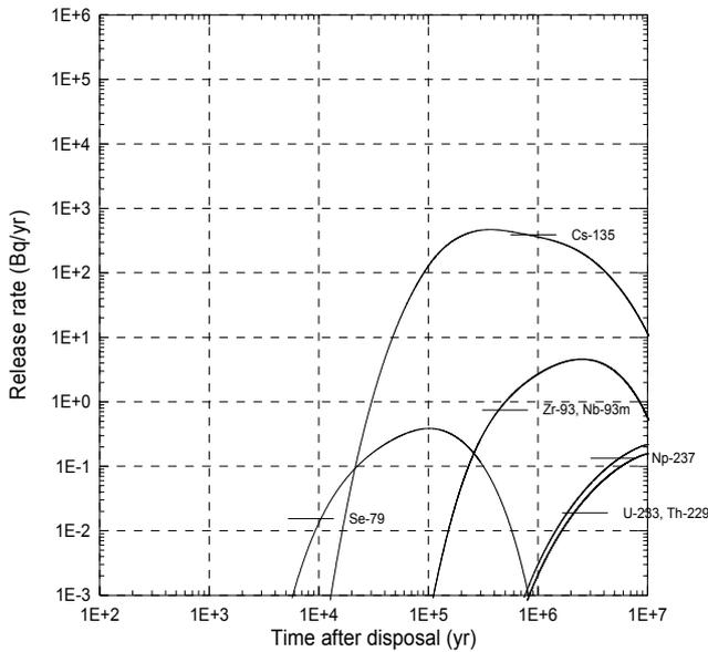
Fig.4 Release rate from the MWCF per waste package
