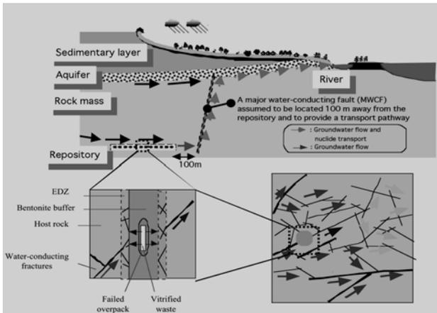
Fig.1. Illustration of the processes considered in the parallel plate model
