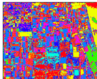
Fig.6 Results of MAP classification using HH channel and K-distribution
