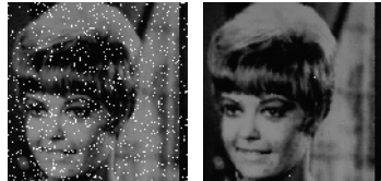
Fig.1.3 Fig.1.4 S/Ni RATIO IS \rightarrow 0.10 dB S/No RATIO IS \rightarrow 1.24 dB ENHANCE FACTOR \rightarrow 1.30 dB
