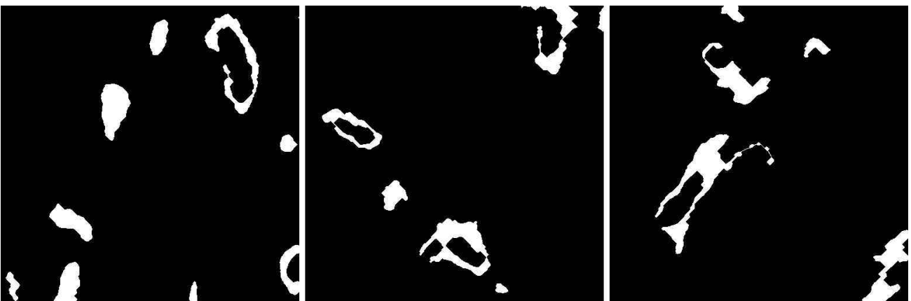
b) Erosion-thinning operation
