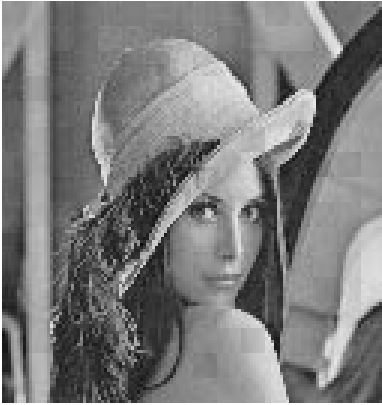
Fig. 13: Simulation result with the increased standard deviation of \sigma = 3\% and an A/C-converter resolution of 10bit
