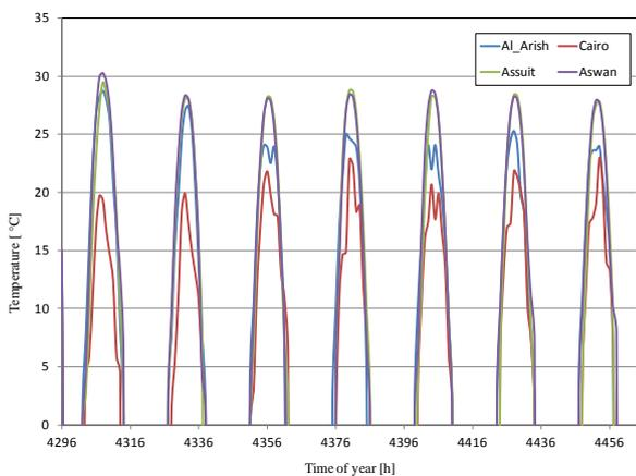
Fig. 3 The collector temperature rise for the selected four cities in Egypt
