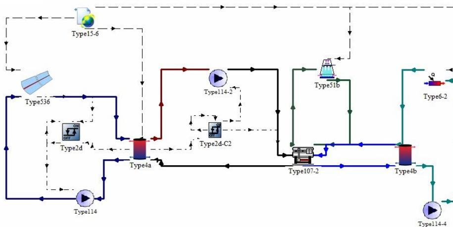
Fig. 1 layout of the TRNSYS simulation model for solar absorption cooling system with PTC
