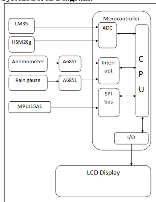
Fig.5 System block diagram
