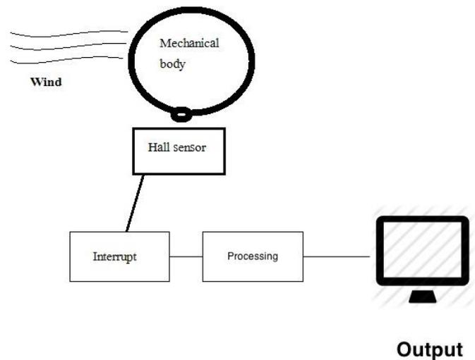
Fig. 2 Block diagram of anemometer
