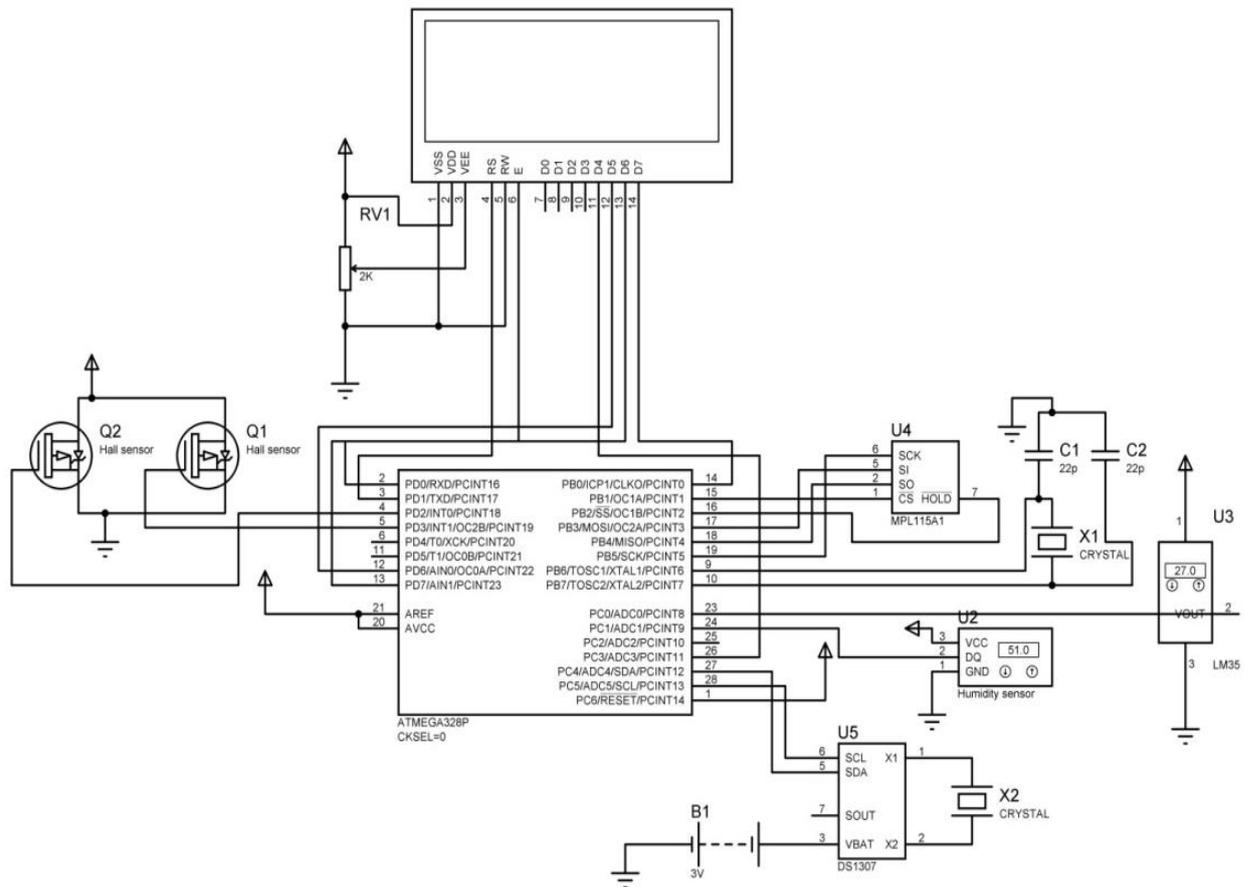
Fig. 6 Schematic of Weather Station
