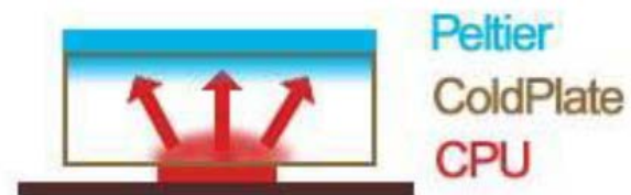
Figure 6: Coldplate to cool a CPU with Peltier.
