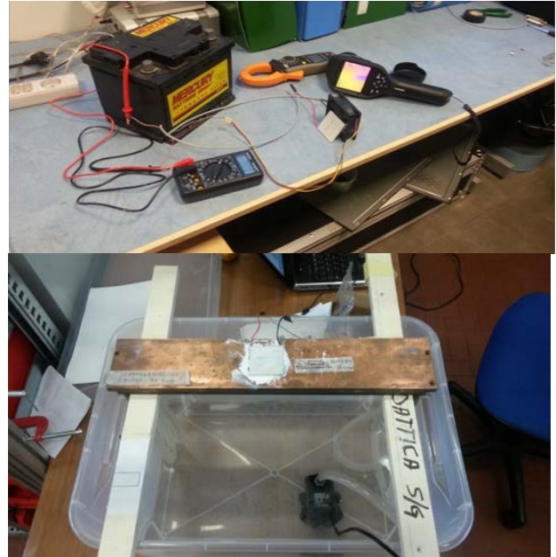
Figure 7: Instrumentation and experimental set-up with Peltier cell, linked to the water heat exchanger.
