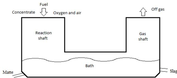
Figure 1: Schematic structure of outotec copper flash smelting furnace
