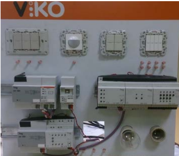
Fig. 4. KNX test panel used in this system.
