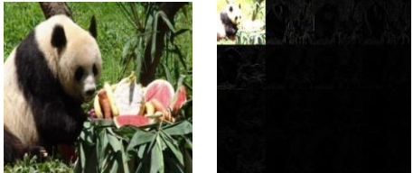
Fig. 2 Original signal and its corresponding wavelet transformed signal. In the right picture, left top part is approximation, others are details.
