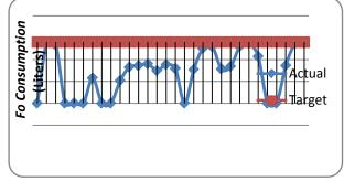
**Figure 16**. Graph of Titan 05Fuel Oil M/E Consumption on Sept 2014
