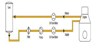
Figure 2. Scheme of flow meter on board
