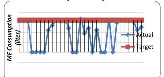
Figure 13. Graph of Titan 03Fuel Oil M/E Consumption on May 2014
