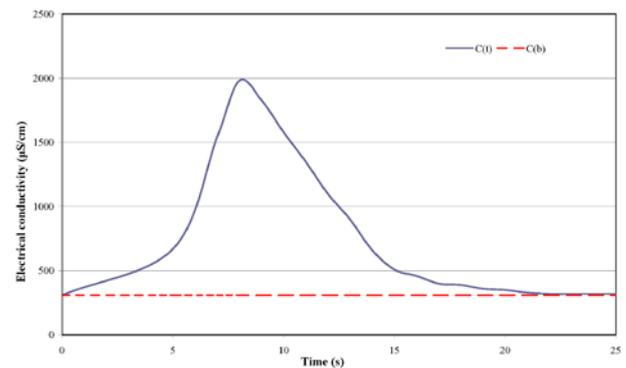
Figure 6 - An example of a salt dilution measurement done at ST\_01
