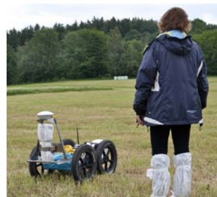
Fig. 4 Orpheus robot during the First experiment. Vital parts were covered by plastic bags as radiation dust protection.
