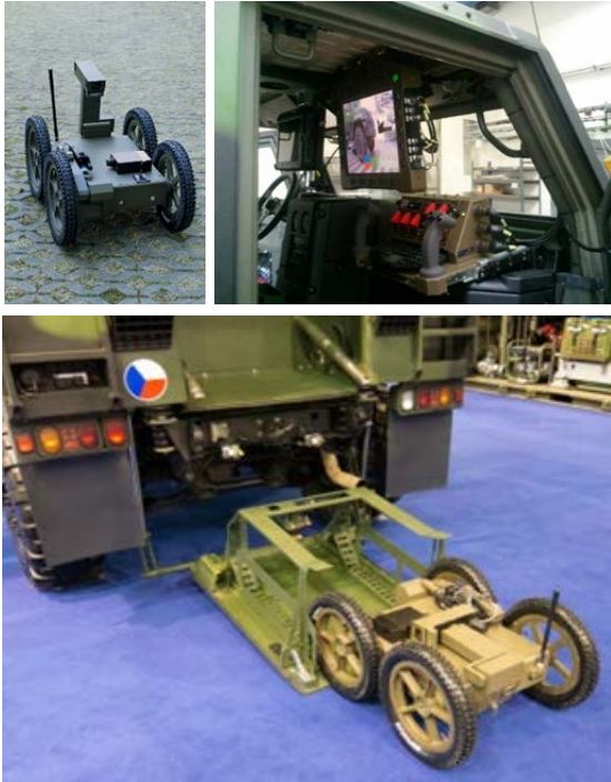
Fig. 1 Orpheus-AC2 military robot for CBRN operator-controlled reconnaissance.
