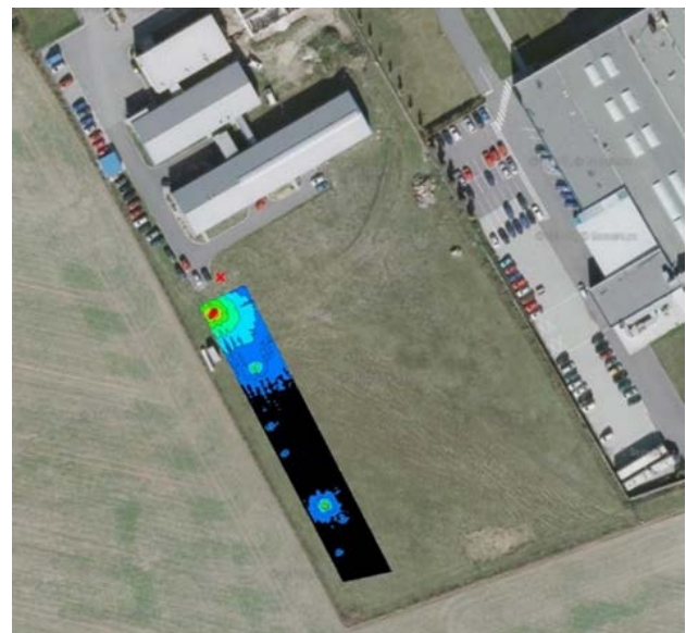
Figure 10. Resulting gamma-radiation diagram in aerial photo (up); demonstration of intensity diagram calculated based on imprecise data from non-RTK GNSS (down).
