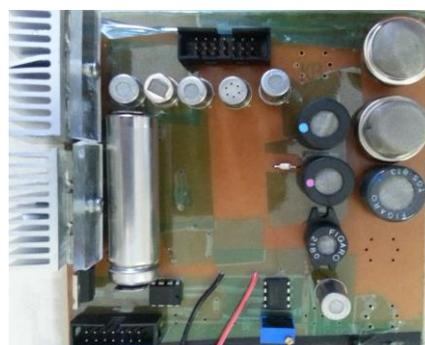
Fig. 1. 13 gas sensor array
