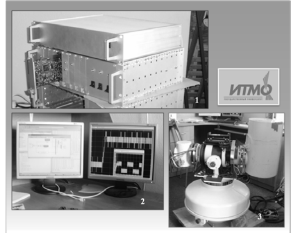
Fig. 4: Laboratory bench of control system prototyping for tracking telescope servo drives.
