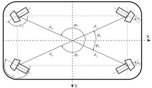
Fig. 3. A configuration of thrusters in subsystem responsible for horizontal motion ( $d_i$  – distance of  $i^{th}$  actuator from centre of gravity,  $\alpha_i$  – angle between longitudinal axis and symmetry axis of  $i^{th}$  actuator,  $\varphi_i$  – angle between longitudinal axis and line connecting centre of gravity with centre of symmetry of  $i^{th}$  actuator).
