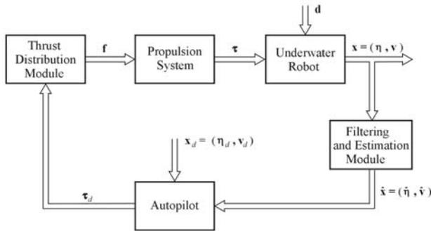
Fig. 1. A block diagram of the control system ( $\mathbf{d}$  – environmental disturbances).
