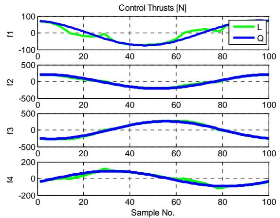
Fig. 6. Thrusts developed by thrusters (L – solution for LP problem, Q – solution for QP problem).
