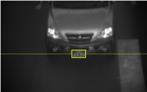
Fig. 6. Estimated plate location which is derived by connected component analysis.
