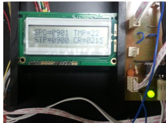
Fig.5. The motor parameters read by the system after the command speed is executed.
