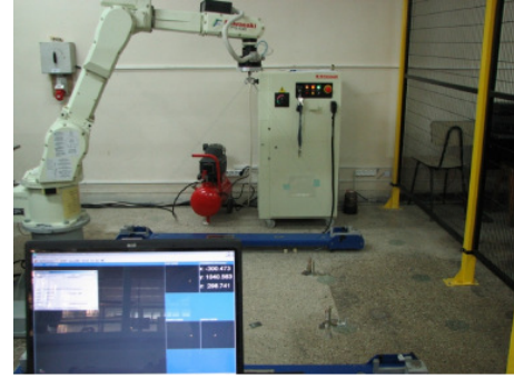
Fig. 3. A measuring setup using Dynalog CompuGauge System
