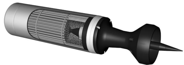
Fig.2: Projectile and travelling charge conjointly.
