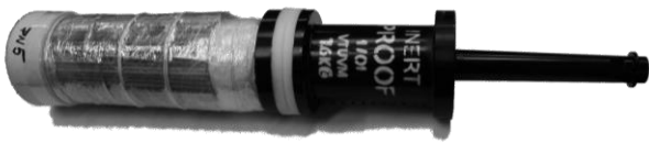
Fig.7: Inert projectile with modified charge.
