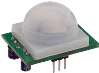
Fig.3: PIR Motion Sensor
