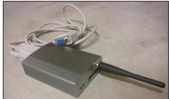
Fig.6: MOD 9001-D GSM/GPRS Modem complete with antenna and RS232 cable
