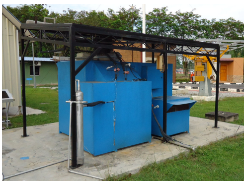
Fig. 5. The photograph of the solar dryer with hybrid PVT-mechanical heat pump
