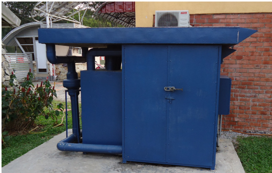
Fig. 2. The photograph of the solar dryer with mechanical heat pump
