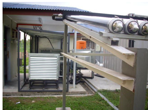
Fig. 15. The photograph of solar dryer with solid desiccant wheel
