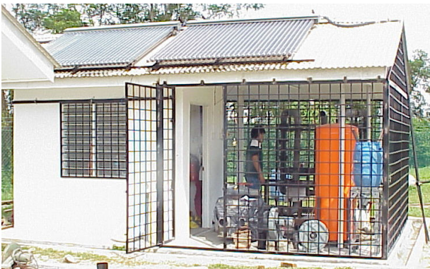
Fig. 13. The photograph of solar dryer with dehumidification system
