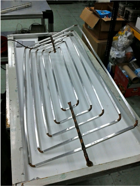
Fig. 5: Thin aluminums are placed to all copper tubes.
