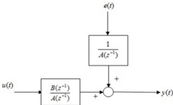
Fig. 3: Model structure of ARX
