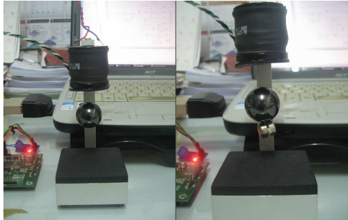
Fig. 4 Proposed magnetic levitation system: (a) without disturbance, (b) with disturbance
