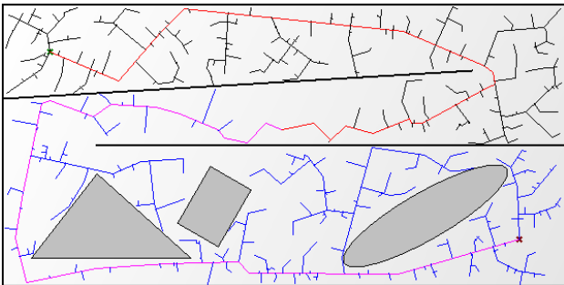
Fig.9: RRT Bidirectional on a maze-type map
