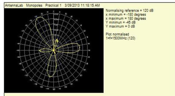
Fig. 15 Monopole radiation pattern
