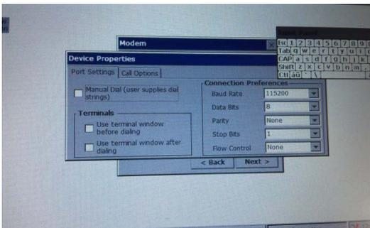
Fig. 10 GSM Modem Configuration
