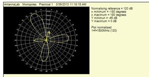
Fig. 6 Monopole Ground Reflection
