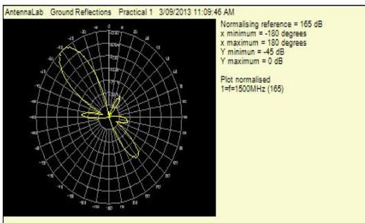
Fig. 3 Ground reflection radiation pattern
