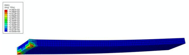
Fig. 26: Concrete plastic equivalent strain from compression, PEEQ=4.88E-3
