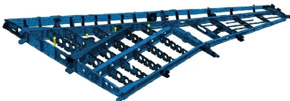
Figure-8: Optimized meshed model of the wing
