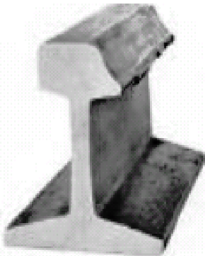
Fig. 5 - Rolling contact forces combined with friction induce wear
