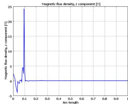
Fig.14 Variation of the Oz component of the magnetic flux density at the media interface for gauge off
