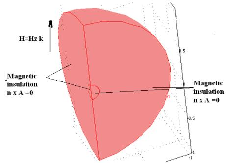
Fig.2 Model and boundary conditions
