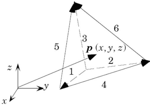
Fig.1 Low order tetrahedral vector finite element
