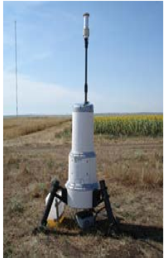
Figure 2. Measurement Equipment LIDAR laser (close-up) and NRG (distant view)
