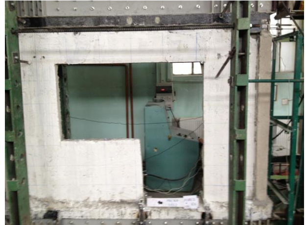
Fig.5 Specimen mounted and ready for testing
