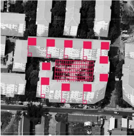
Fig.8 Solar thermal and PV systems
