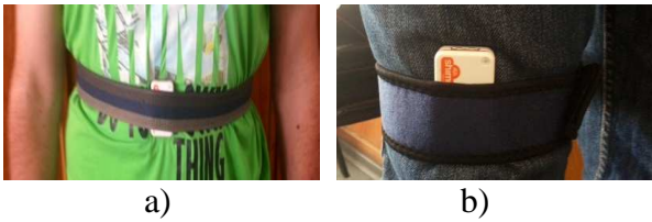
Fig. 9. Accelerometer placement: a) torso, b) leg
