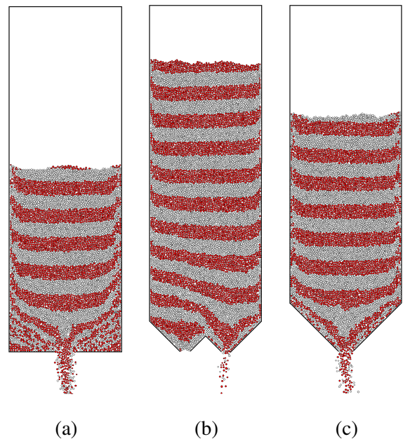
Figure 6: Effect of the hopper shape on discharge pattern at t = 75 s : (a) a flat-bottomed silo; (b) a silo with double-opening bottom and (c) a cylinder-hopper silo.
