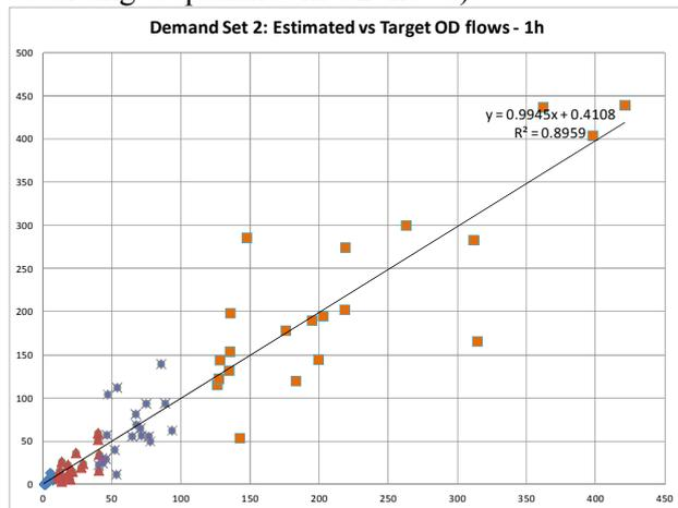
Figure 3. Fit estimated KFX versus Target OD flows. 100% BT equipped and reliable initial OD matrix. Detection layout reduced to 50%
