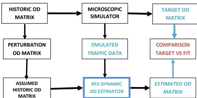
Figure 1. Methodological Design Of The Experiments By Simulation
