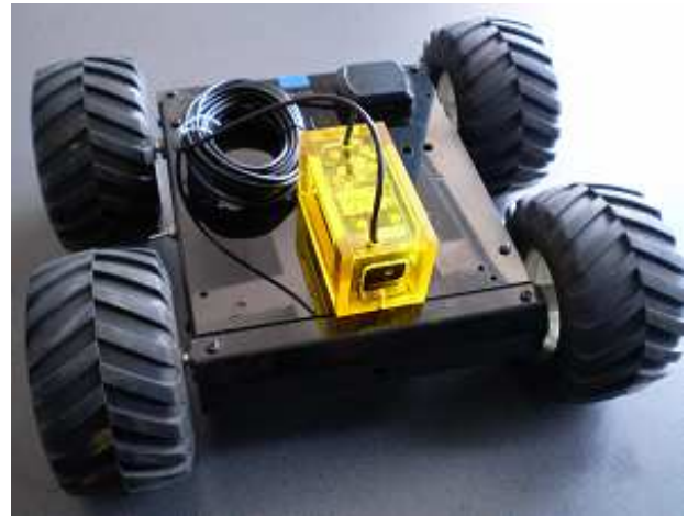
Fig.3. Mobile platform equipped with wireless sensor and GPS antenna.
